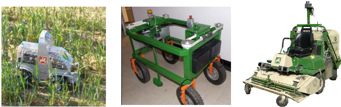
Fig. 1: Concepts for the development of autonomous field robots: Experimental approach Field Robot Event (left side, field robot Maizerati [4]), new design of autonomous field robots (centre, autonomous robot WEEDY [3]), automation of existing vehicles (right, Profihopper)
