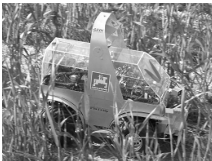
Fig. 7: Autonomous field robot Maizerati (KLOSE et al. 2007), which has been designed for the Field Robot Event.
