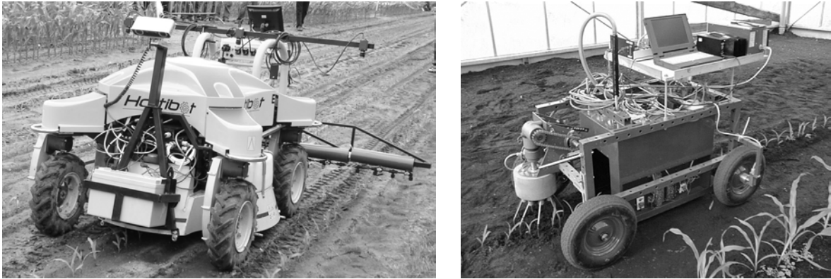
Fig. 5: Left side: HortiBot (Aarhus University, Danish Technological Institute, Vitues Bering Denmark; photograph: A. Ruckelshausen, Field Robot Event 2007 in Wageningen/The Netherlands; JØRGENSEN et al. 2006). Right side: Mobile sensor unit with a sensor-based cycloid hoe (“Querhacke”) in greenhouse experiments (University of Applied Sciences Osnabrück, RUCKELSHAUSEN et al. 1999; supported by the Deutsche Bundesstiftung Umwelt).
