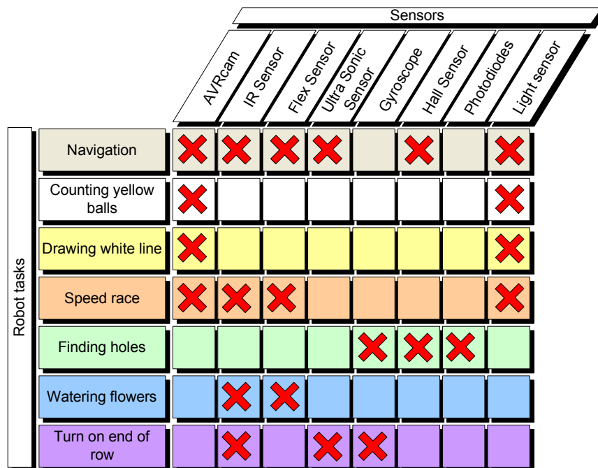
Figure 3: Sensor fusion concept of the autonomous field robot Maizerati for the Field Robot Event 2006
